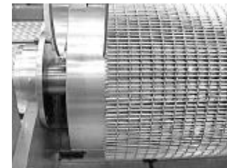
Fig. 3 — Type T.N.E/PS loom for architectural fabrics & transport belts (inset: close-up of woven product).
