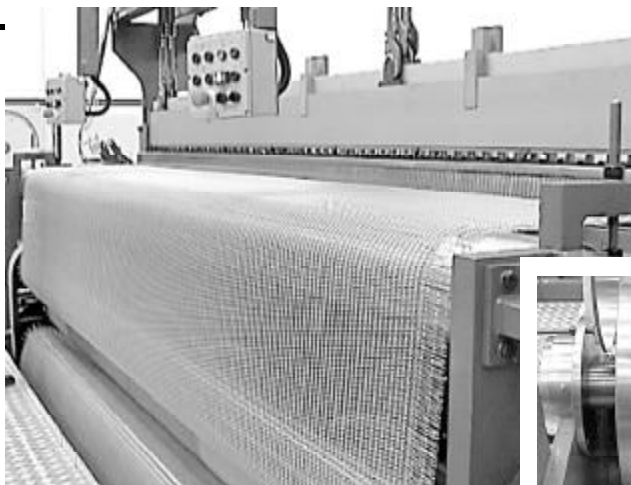
Fig. 3 — Type T.N.E/PS loom for architectural fabrics & transport belts (inset: close-up of woven product).
